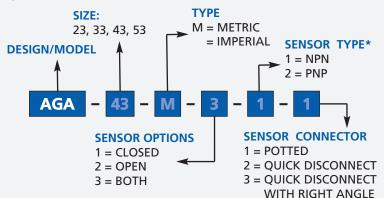
\* NOTE: Hall Effect 4mm dia., 5-24 VDC, 22 mA and comes with 2 meter
