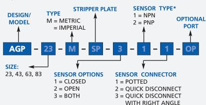
\* NOTE: Hall Effect 4mm dia., 5-24 VDC, 22 mA and comes with 2 meter cable.
