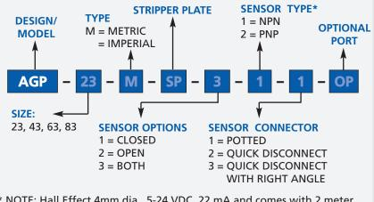
\* NOTE: Hall Effect 4mm dia., 5-24 VDC, 22 mA and comes with 2 meter cable.
