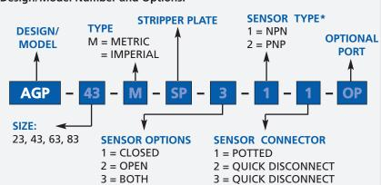
\* NOTE: Hall Effect 4mm dia., 5-24 VDC, 22 mA and comes with 2 meter
