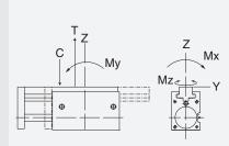
Static **Dynamic** Max Tensile T 250 lbs 108 lbs [1112 N] [800 N] Max Compressive C 250 lbs 108 lbs [1112 N] [800 N] Max Moment M<sub>x</sub> 120 in/lb 62 in/lb [8 Nm] [7 Nm] Max Moment M<sub>v</sub> 120 in/lb 62 in/lb [8 Nm] [7 Nm] Max Moment M<sub>7</sub> 120 in/lb 62 in/lb [8 Nm] [7 Nm]
