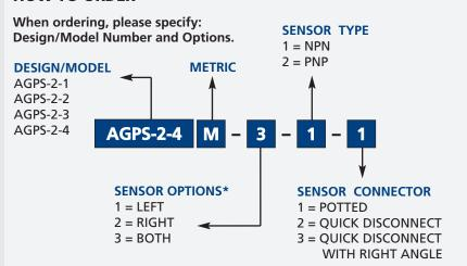
\* NOTE: Hall Effect sensors are hard wired with 20"pigtail.
