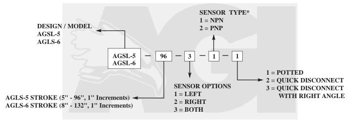
\* **NOTE:** Proximity sensors are 8 mm dia., 12-30 VDC, 200 mA and come with 2 meter cable. Sensor Part# SNC08, SNQ08, SPC08, SPQ08
