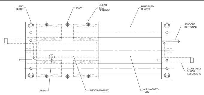
• Magnetically coupled cylinder is designed to be leak free due to no mechanical connection between the piston and the body.
