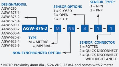
\* NOTE: Proximity 4mm dia., 5-24 VDC, 22 mA and comes with 2 meters cable.
