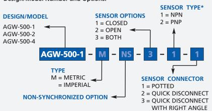
\* NOTE: Proximity 4mm dia., 5-24 VDC, 22 mA and comes with 2 meter cable.
