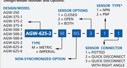
\* NOTE: Proximity 4mm dia., 5-24 VDC, 22 mA and comes with 2 meter cable.
