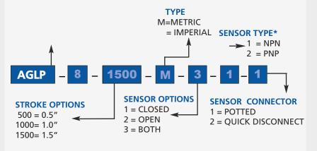
\* NOTE: Hall Effect 4mm dia., 5-24 VDC, 22 mA and comes with 2 meter cable or quick disc.
