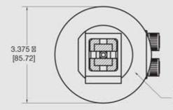
ORIENTATION SHOWN AT HOME POSITION UNIT ROTATES CLOCKWISE PER THIS VIEW
